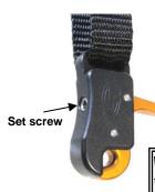
Using a 3/32 hex key, turn set screw clockwise to decrease tension (toward hair-trigger) & counter-clockwise to increase tension.
