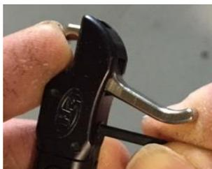
While pushing on the jaw with your finger, turn the set screw slowly clockwise until the jaw opens. Then turn the set screw counter-clockwise 3/4 turn. This is the most sensitive setting that is safe to shoot.
