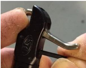
While pushing on the jaw with your finger, turn the set screw slowly clockwise until the jaw opens. Then turn the set screw counter-clockwise 3/4 turn. This is the most sensitive setting that is safe to shoot.
