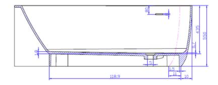
Net Weight: 105kg Gross Weight: 155kg Water Capacity: 270L Unit: mm
