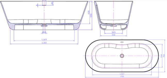
Net Weight: 115kg Gross Weight: 165kg Water Capacity: 240L
