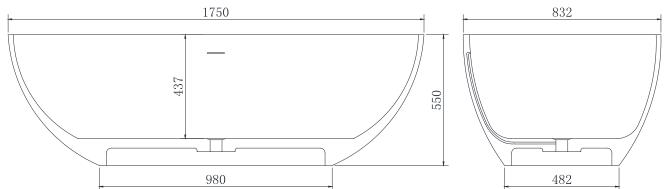
Net weight: 167kg Gross weight: 239kg Water capacity: 300L Unit: mm
