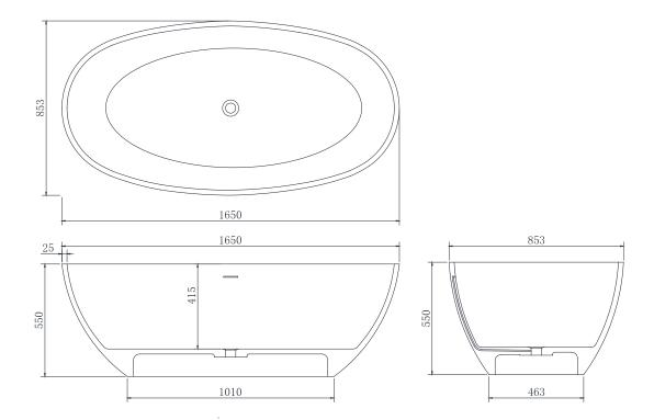
Net weight: 168kg Gross weight: 238kg Water Capacity: 255lt
