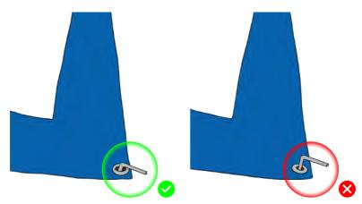
Next, if feasible, secure the Pause Box to the ground by anchoring it with 4 pegs (B), one at each designated corner.
