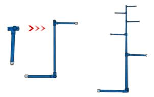
Next, attach the other end of the Intermediate base pole (E) in a zig-zag configuration with a Tee-Shaped base pole (F).
