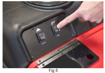
7. Turn vacuum switch to the "on" position to begin cleaning. (Fig 6)
