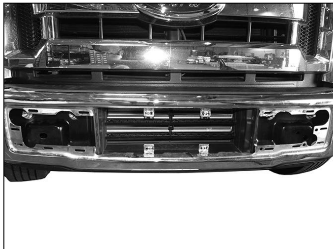
(Fig 2) Remove license plate. From behind bumper, release metal clips attaching plastic bumper pad to the bumper
