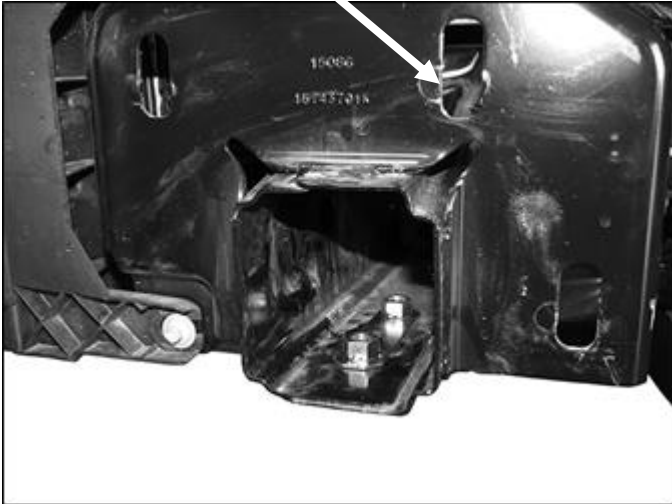
(Fig 5) Reuse factory double nut plate (models with tow hooks) or insert included Double Nut Plate into end of frame
