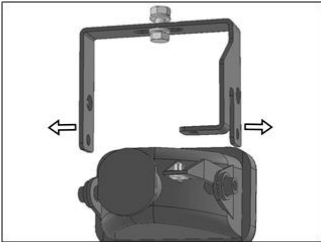
(Fig 13) Carefully spread sides to slide OEM fog light into position in pivot holes
