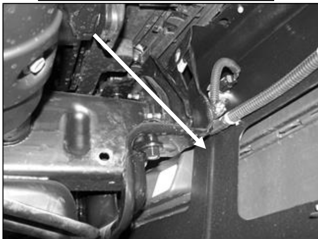
(Fig 1) Unplug wiring harness and move it away from bumper before removal
