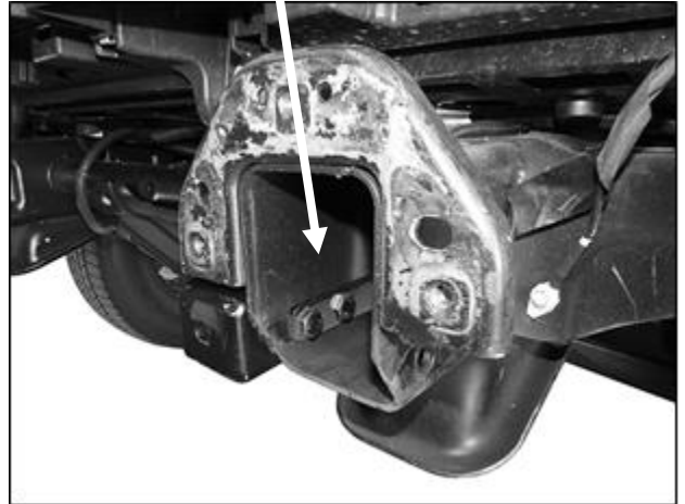
(Fig 7) Driver/left side of frame with Right Facing Support Bracket installed
