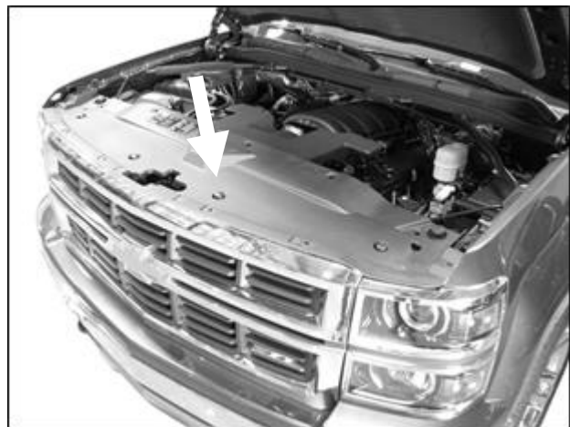
(Fig 3) All models years, remove plastic cover from top of radiator (arrow). Temporarily remove grille
