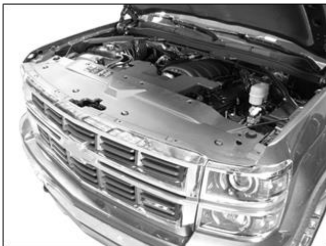
(Fig 2) On 14-15 models, from behind bumper, release clips and hardware attaching plastic fascia panel (arrow) to top of bumper and fenders. Remove fascia panel to access grille and bumper hardware from above.
