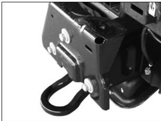
(Fig 4) Remove inner bumper brackets and tow hooks, reinstall plastic grille and cover
