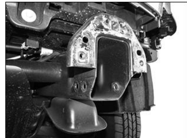
(Fig 5) Bumper, tow hooks and brackets removed
