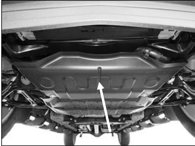
(Fig 7) Diesel equipped only: Remove forward splash guard (arrow)
