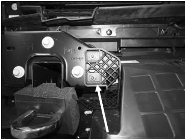
(Fig 9) Diesel equipped only: Remove the bolts and pins attaching the shroud to the vehicle (arrow). Unplug and remove shutter assembly
