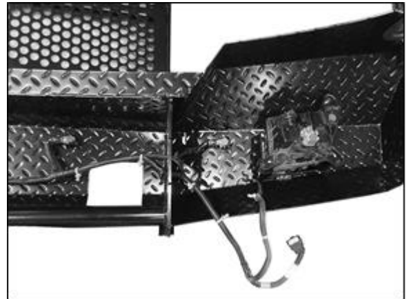
(Fig 27) Install wire harness. Use Harness Extensions to reach sensors as needed
