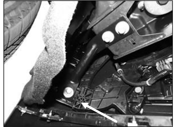
(Fig 4) Remove outer bumper supports (arrow)
