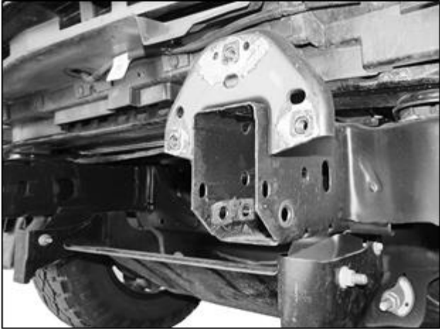
(Fig 11) Brackets and tow hooks removed
