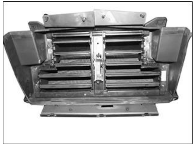
(Fig 10) Diesel equipped only: Remove the shutter assembly from the outer housing
