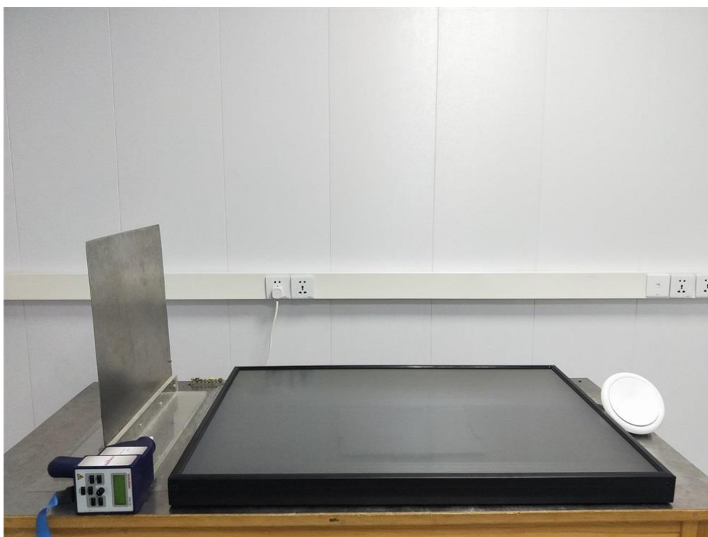
Test Setup Photo of Electrostatic Discharge Test
