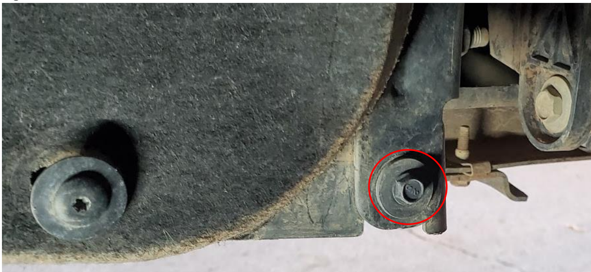
Figure 3 7mm Hex Bolt
