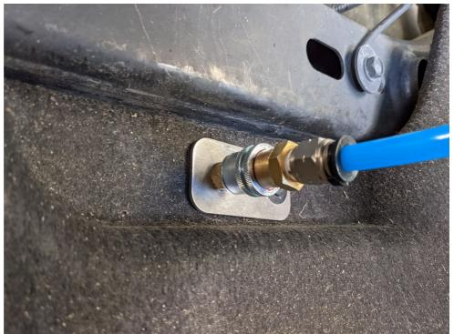
11. Open the hand slide valve with all four corners connected and let
