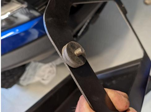
18. Put one rubber washer on each of the other studs on the tray, including the two on the bottom of the battery tray.
