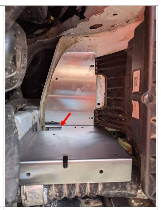
15. Reconnect the horn, and reinstall the trimmed fender filler panel. There is a hole for the OEM wire mount provided on the bracket.
