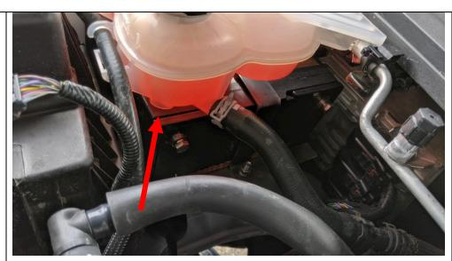
29. The final step of the install takes some trial and adjusting to find the "sweet spot" where the coolant tank doesn't contact the hood.
