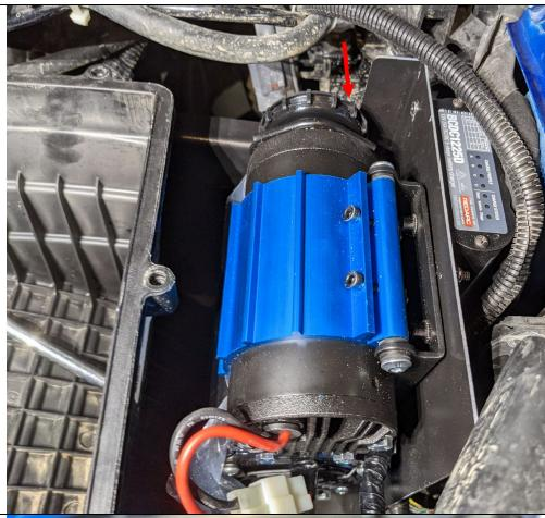
12. Using three more of the supplied ¼" nuts and lock washers, secure the upright bracket to the base via the 3 studs. There are two vertical studs on the bottom and one horizontal stud near the top.
