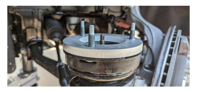
15) Reinstall the shock into the vehicle
