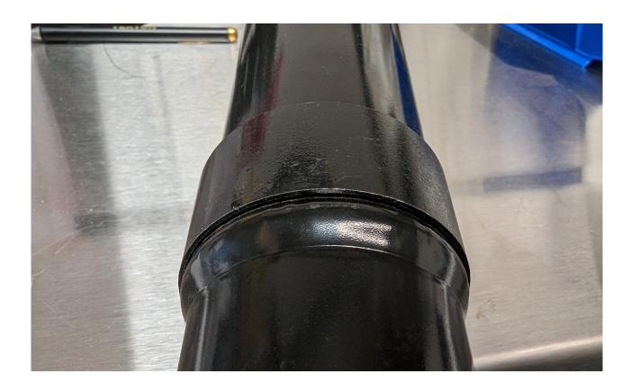
12) Place spring seat onto shock and shock spacer making sure it is fully seated
