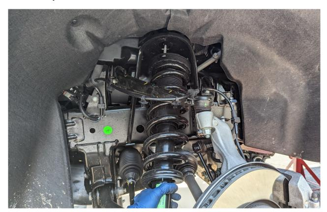
10) Using a spring compressor, compress the spring and remove the upper mount, pay close attention to the upper mount orientation, it is best to mark it relative to the shock to make reassembly easier 11) Place provided shock spacer over the shaft and onto the
