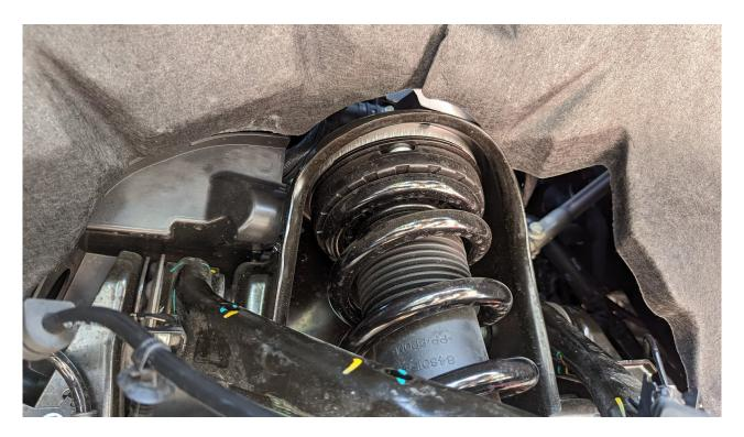
13)Install the provided hardware using 15mm ratcheting wrench
