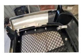
6- The OKF grille is installed. Now it is time to reinstall on the vehicle.
