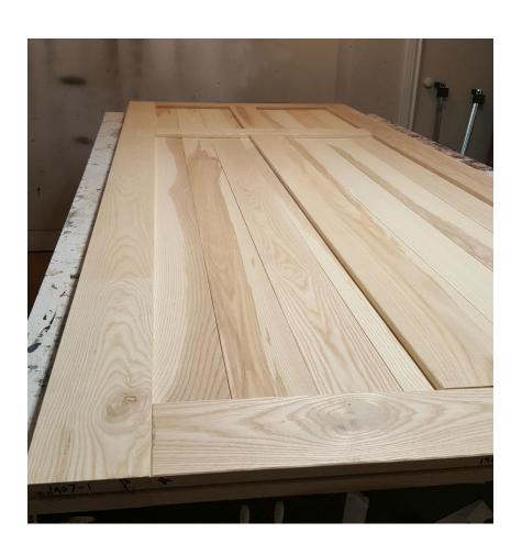
Shoot your screws in and the door will be fully assembled. The holes for your hardware are already drilled at the top.
