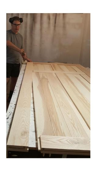
When you install the second vertical piece you will need to start at the top. Align the joint and then tap it together with a rubber mallet.
