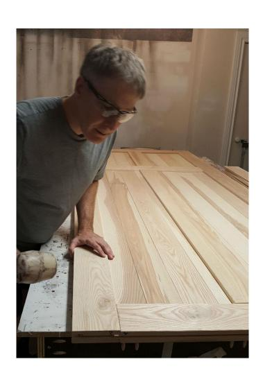
You will need to tap the bottom together with a rubber mallet, and may need to tap the bottom horizontal to get it to perfectly line up.
