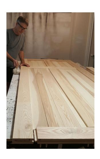
Continue to tap the vertical side moving down the door, thus closing the gap at the bottom of the door.
