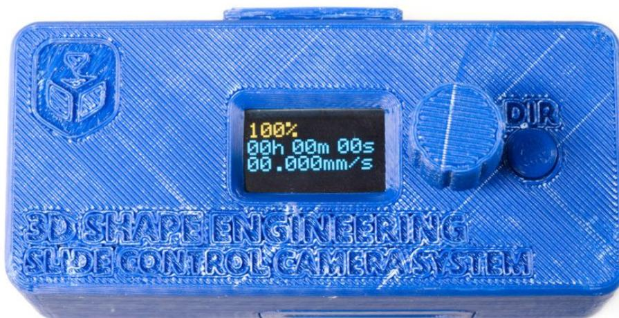
The lcd screen is used to display battery life, movement speed (in millimeters a second), the amount of time it will take to move across the entire length of the slider as well as the current state of the motor movement.
