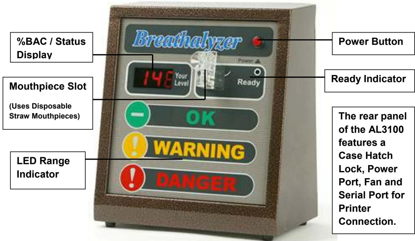
The AlcoScan AL3100 is a table-top wall-powered breathalyzer that measures a breath sample to detect alcohol in the lungs. The reading is converted to blood alcohol concentration (BAC). The AlcoScan AL3100 uses an advanced semiconductor sensor to detect alcohol. The AL3100 uses Pre-Calibrated Replaceable Sensor Modules to eliminate the need for calibration. The sensor module should be replaced approximately once every 500 tests.
