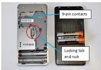
Remove the rear cover, then remove the batteries. Use your finger to hold down the small tab highlighted to the left, and pull the sensor module straight down. You can then simply lift the module up from the device.
