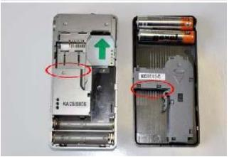
To install a new sensor module, place the portion of the sensor module highlighted to the left flush against the section of the slot also highlighted. You can then simply slide the sensor module up into place, as shown by the green arrow. Ensure the tab is locked in place against the small gray locking nub near the center of the device.
