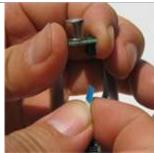
Remove the cable from the slot underneath the sensor module.
