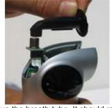
Remove the breath tube. It should remove easily
