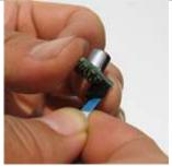
Insert the cable into the new sensor. Make sure the blue strip is toward the sensor, as shown.
