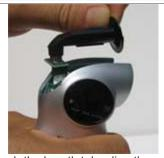
Re-attach the breath tube directly on to the sensor. Make sure the front opening is aligned.
