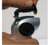
Lift the breath tube to access the sensor module.
