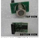
Prepare a new pre-calibrated sensor module.
