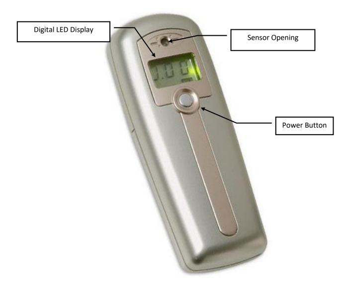
The AlcoScan AL2500 analyzes a breath sample to detect alcohol in the lungs. This reading is then converted to blood alcohol concentration (BAC). The AlcoScan AL2500 is very convenient and portable. No mouthpiece is required.
