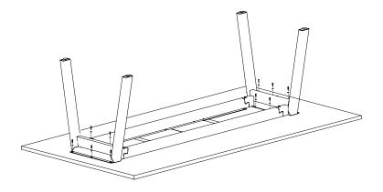
With a buddy, flip the table back over. Adjust leveling feet until all feet lay flat on the floor.
