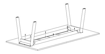
Fully secure the frame to the table top using the remaining wood screws and washers.
