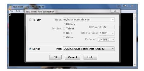
3: Select the "Serial" button and choose the correct COM port for your USB/Serial cable. In this case our computer used COM 43. Your computer may assign a different COM port.
