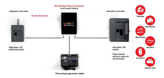
An additional 3-phase breaker panel may be installed on the line between the converter control panel and the 3-phase equipment. This is recommended to protect each piece of equipment and the wire that feeds that equipment.
