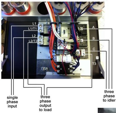
The following diagram shows the electrical schematic for the rotary phase converter:
