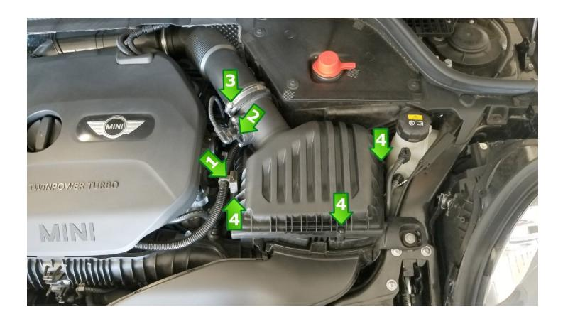
5. Attach the billet bracket to the lower air box lid below using one of the factory torx screws. Make sure secure and positioned exactly like the photo below.
