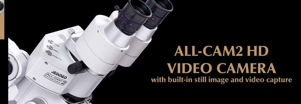
The ALL-CAM2 utilizes a continuous 1080P 60FPS HD video sensor. The real-time image output and all capturing is full 16:9 high definition. All controls are conveniently located and executed at the touch of a button. Still images and video recordings are captured directly to a USB disk. All files are Hi-Def digital and can be easily transferred via USB disk as jpeg and MP4.
