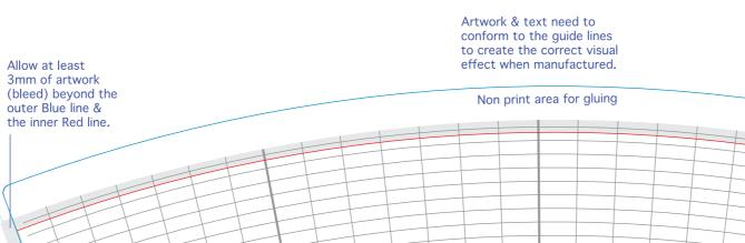
Outer Blue line indicates the cutting form shape of the cup.
