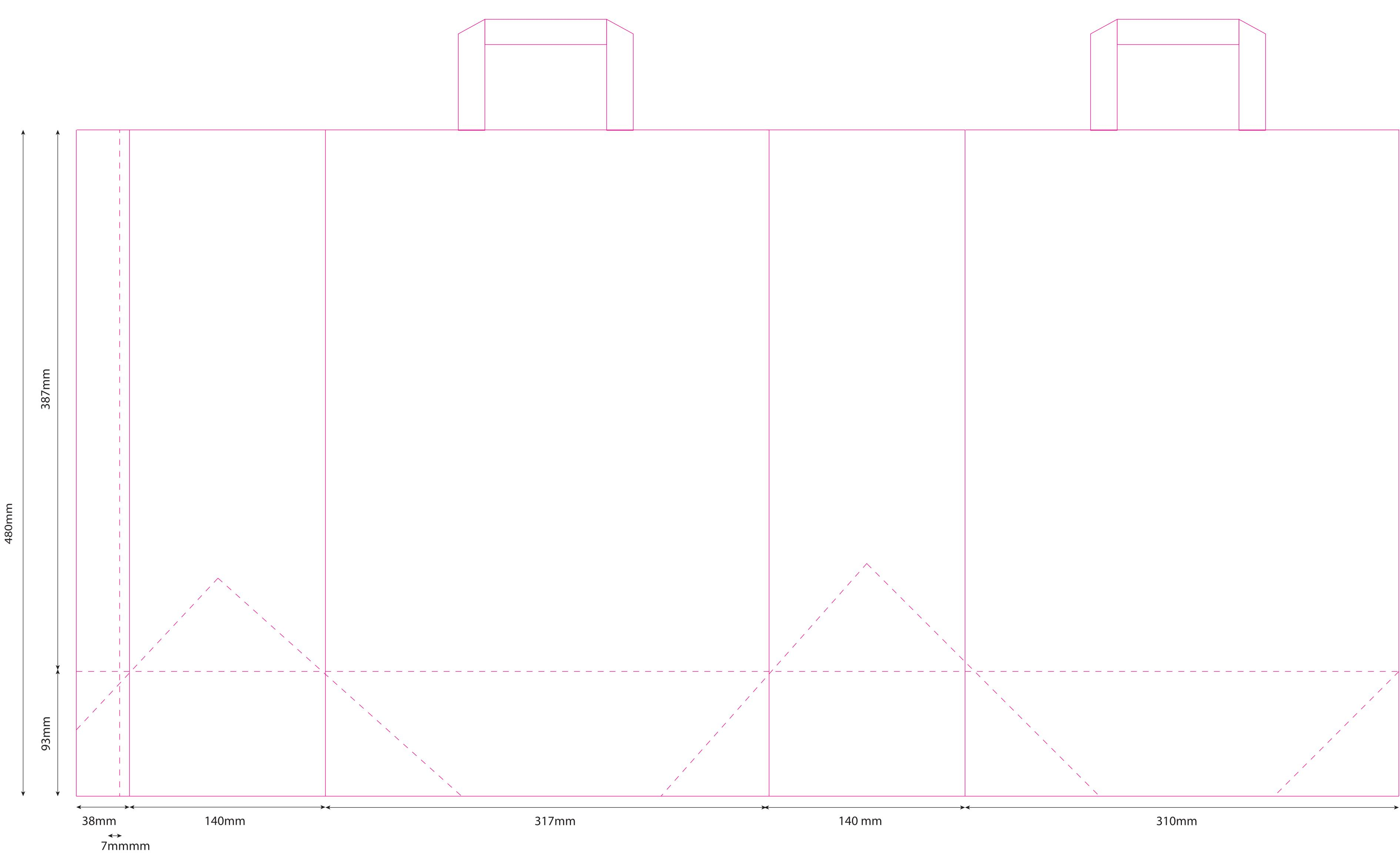
An extra 4mm of print is required on the left hand edge if design wraps around to the reverse. If there is solid print in the gussets, please pull the print in by 1mm either edge. If there is solid print on front/reverse, please add 1mm bleed into either gusset.
