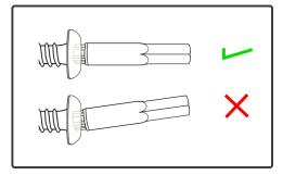
Make sure when driving your screws in that the bit is lined up straight with the screw to ensure a clean installation and avoid potential stripping or breakage of the screw or bit.
