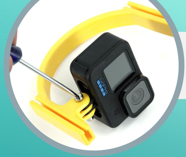
Make sure the camera is angled correctly. Take a screwdriver and tighten the bolt as much as possible, the camera should now not be able to move.
