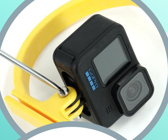
Slide the bolt into the mount, hold the nut in the recess, finger tighten the bolt.
