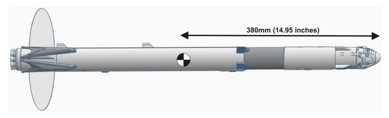
Failure to adjust the models C.G. to the position shown will result in a unstable flight that could injure someone, damage personal property and damage or destroy your model.
