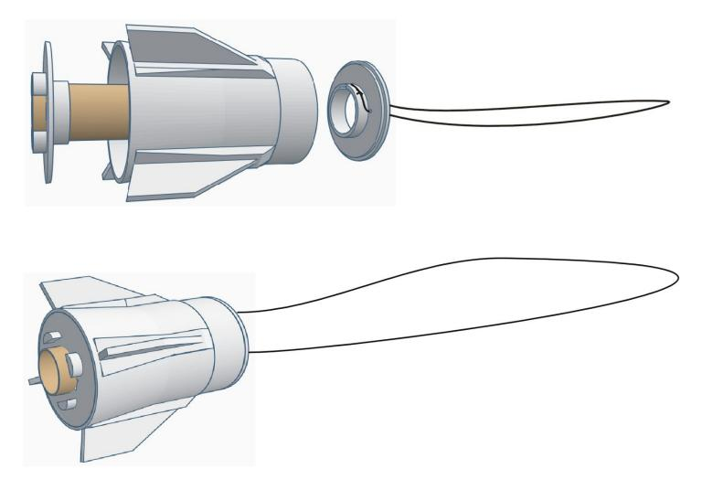
Attach an elastic shock cord roughly 36" long (915mm) to the forward loop in the Kevlar shock cord anchor. We prefer 1/4" (6.35mm) braided elastic.
