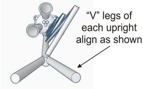
After all 3 uprights are seated and aligned apply super glue to each cross member/upright joint and hold till dry. Repeat for each upright.
