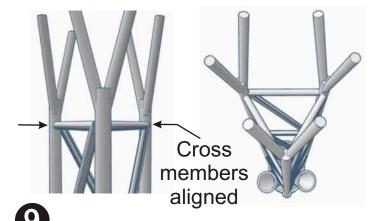
Carefully flip the tower assembly over and insure each upright is fully inserted into its hole in the nozzle assembly. Apply a drop of super glue to the top of each tower upright through the holes.
