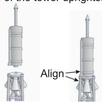
Sand the capsule and primer as described above. Paint the capsule flat black. When dry super glue the tower on as shown.
