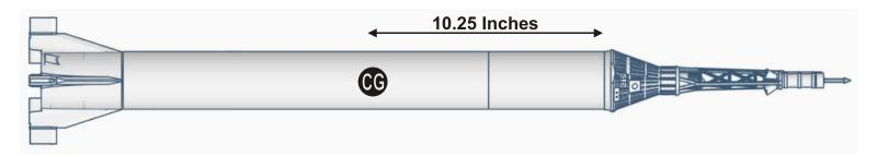
Please note that this procedure must be repeated if you use a larger/heavier rocket motor on later flights. Failure to correct the models center of gravity may result in an unstable flight which can damage or destroy the model and cause harm to personal property and human life.
