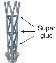
After the tower is dry, check it for vertical trueness on each of its 3 sides. Carefully sand the base legs of the tower to adjust trueness if needed.
