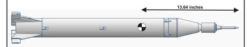
Failure to adjust the models C.G. to the position shown will result in a unstable flight that could injure someone, damage personal property and damage or destroy your model.
