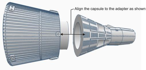
Sand the coupler/shoulder until the shoulder is a nice slide fit in your BT-80 body tube. Determine the amount of nose weight you need to add to the capsule to insure a stable flight. Add nose weight using epoxy and small lead fishing weights or clay Into the space provided in the capsule. Make sure you leave enough room to insert the coupler/shoulder completely. When the nose weight is dry glue the tube shoulder to the capsule section using either super glue gel or plastic epoxy.
