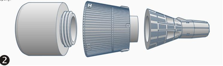
Tie a large two foot piece of 150 lb test Kevlar cord to the base of the capsule coupler/shoulder. Add a short length of shock cord and a 36" parachute or other recovery system as desired.
