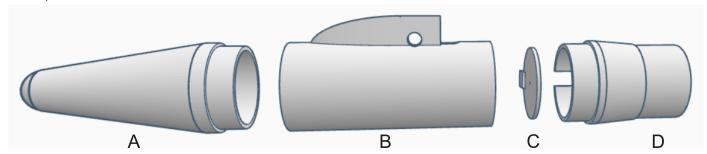
Check the fit of the nose cone (A) into the top of the payload tube (B) and the fit of the lower transition (D) into the bottom of the payload tube (B). Sand with 220 sandpaper if needed to ensure a nice slip fit into each other. Before assembly screw and super glue the provided metal screw eye for your recovery system into the outside hole in the base of the lower transition (D).
