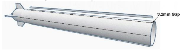
7. Attach the launch lugs. The launch lugs are, of course, located on the launch lug line. Mark this line ¼" (6.4mm) and 9" (228.6mm) from that AFT end of the body tube. Attach the launch lugs with their aft ends at these marks using CA glue, making sure the launch lugs are aligned. Apply CA or epoxy fillets to the launch lug/body joints. Allow to dry.
