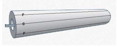
5. <u>Assemble the fins</u>. Glue one main fin on each of the fin lines. The plastic piece at the bottom of each fin (a fixture the actual missile rests on, when it is upright on the launch table) will sit up against the aft centering ring (apply glue to this joint, as well as the fin/body tube joint). Make sure the fins are straight when drying. Apply CA or epoxy fillets to the fin/tube joints. For scale accuracy, the fillets should be thin – just for added strength.
