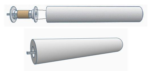
4. Mark the body tube. Place the body tube (aft end down) on the fin location guide. Mark the fin locations, the launch lug location, and the conduit locations. We recommend marking the fin locations with an "F," the launch lug location with an "L," and the conduit locations with a "C." Using a straight edge, extend the fin marks about 4" (~102mm) along the tube. Extend all lines the entire length of the body tube.
