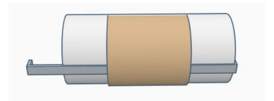
The forward centering ring has a built-in motor block and attach points for a shock cord. Using cyanoacrylate (CA) glue, or "super glue," glue this ring to one end of the motor tube. Glue the other ring to the aft end of the motor tube, flush with the end of the tube. Apply fillets, if desired, to the tube/ring joints and allow to dry.
