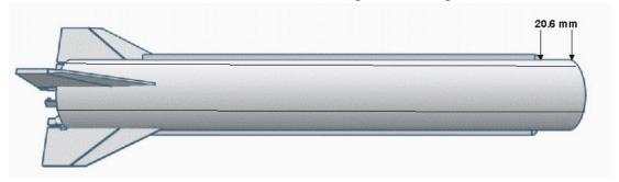
7. Attach the launch lugs. The launch lugs are, of course, located on the launch lug line. Mark this line ¼" (6.4mm) and 6.5" (165.1mm) from that AFT end of the body tube. Attach the launch lugs with their aft ends at these marks using CA glue, making sure the launch lugs are aligned. Apply CA or epoxy fillets to the launch lug/body joints. Allow to dry.
