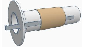
The motor mount is designed to use a Kevlar anchor. 100-pound Kevlar works well. The length should be approximately 36" (915mm). Thread both ends of the Kevlar through the holes in the forward centering ring. Tie a double knot or even a triple knot in the Kevlar so it can't be pulled back through the holes, and use CA to glue it in place. Seal the holss in the ring with CA as well. At the other end of the Kevlar, make a loop about 1" in diameter.
