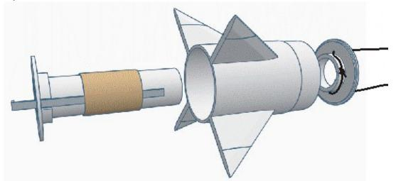
Attach an elastic shock cord roughly 36" long (915mm) to the forward loop in the Kevlar shock cord anchor. We prefer  $\frac{1}{4}$ " (6.35mm) braided elastic.
