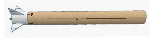
4. <u>Attach the cable conduits</u>. Mark the "C" lines 5/8" (15.9mm) from the front end of the tube. Glue one conduit on each conduit line, with the front end of the conduit at the 5/8"/15.9mm mark. Make sure the conduit is straight along the tube. It should be parallel with the sides of the body tube.
