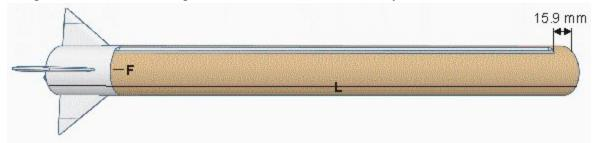
5. <u>Attach the launch lugs</u>. Using a straight edge, extend the "L" line to the bottom of the fin can. Mark this line 1/4" (3.2mm) and 9" (228.6mm) from that AFT end of the <u>fin can</u>. Attach the launch lugs with their aft ends at these marks using CA glue, making sure the launch lugs are aligned. The aft lug is attached to the fin can. Apply CA or epoxy fillets to the launch lug/body joints. Allow to dry.
