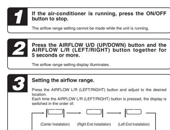
The air-conditioner's airflow range is set. Press within 60 seconds of setting the airflow range (while the airflow range
