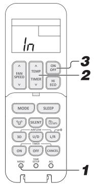
Select the Wireless LAN communication setting by pressing the MENU switch.
