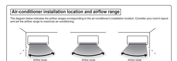
Once the airflow range setting is configured, it is stored in the air-conditioner even if the power source is turned off. To change the airflow range setting, set range again with the remote control.
