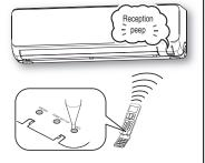
Check that the reception buzzer sound "peep" is emitted from the indoor unit.
