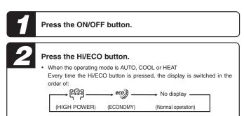
When the operating mode is DRY or PROGRAM TIMER Every time the Hi/ECO button is pressed, the display is switched in the order of:
