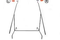
units (F) by inserting the appropriate with corner units (E+F) by inserting them into the connection outlets of the lower diagonal bars(D).
