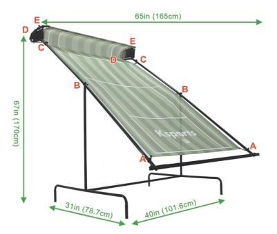
Step 8: Strap up the net between the holes and anchor points along the frame using the bungee loops as shown in the pictures here positions A, B, C, D & E. The Bungee loops should be strapped around the bars to obtain the correct tension on the net.
