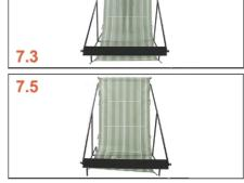
7.2-7.5: Insert the upper horizontal bar through the top of the net (K) if necessary and connect it to each end of the corner units (F).
