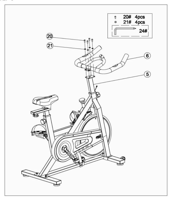
The Handle Frame (6) is fixed on the Handle Post (5) with the Spring Washer (21) and the Round Head Bolt (20) and tightened with the Hexagon Wrench (24).
