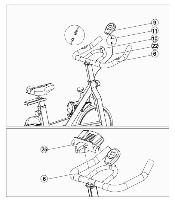
Install the Monitor (9) on the Monitor Holder (10) as shown in the picture and slide the monitor on in the direction of the upper opening of the holder. Tighten the screw on the lower part of the holder with the inner hexagon wrench.
