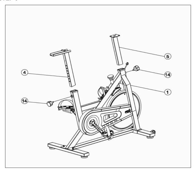
Similarly, the Handle Post (5) is inserted into the Main Body (1), and when the Adjusting Knob (14) is pulled, you can adjust the height of the handles by inserting it into the corresponding hole of the Handle Post (5). The Adjusting Knobs (14) are installed in front and back of the Main Body (1) respectively.
