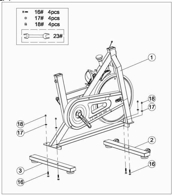
The Front Stabilizer (2) is fixed on the Main Body (1) with Carriage Bolts (16), Flat Washers (17) and Cover Nuts (18) and fixed with Open Spanner (23).
