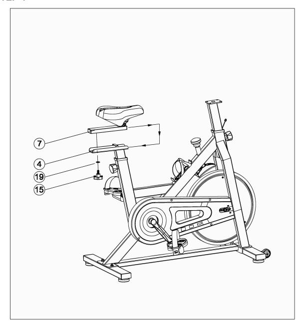
The Seat Adjustment Frame (7) is installed on the Seat Post (4) and is fixed with a Flat Washer (19) and an Adjusting Nut (15).
