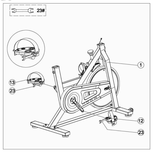
Install the right pedal (12) with R mark on The Main Body (1) and tighten with Open Spanner (23).
