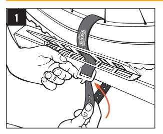
With the buckle's prong facing upward, wrap the strap around the wheel and the rack then feed the end through the buckle.
