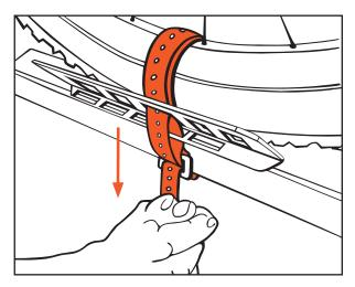
Wrap the strap 2X around the wheel and rack for extra security on long trips or driving off-road Bend the strap back onto itself, then pull it tightly until you find the best hole for the prong.
