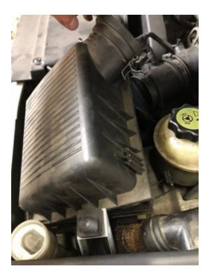
Once the lid is removed, pull up on the power steering reservoir and push out of
