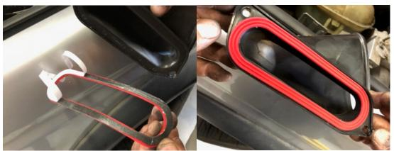
\*Please note second gasket is for when you are installing a snorkel at the outer fender position.
