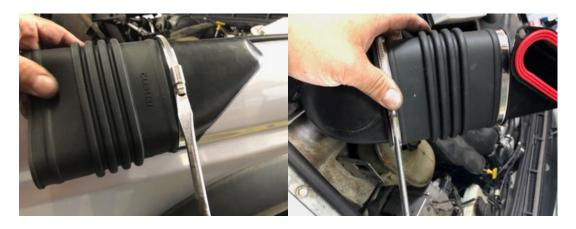
\*PLEASE NOTE! IF YOU PLAN ON CROSSING WATERWAYS WE SUGGEST ADDING A SMALL BEAD ON SILICONE SEALANT AT BOTH SILICONE TUBE ENDS TO PLASTIC JUNCTIONS BEFORE TIGHTENING CLAMPS.
