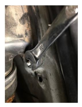
Be very cautious not to molest the small line going into the radiator at the top position shown here, if it is bent it can break the small plastic nipple on your radiator, that's no Bueno.
