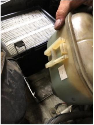
Now pull up on lower airbox assembly to remove entire unit.
