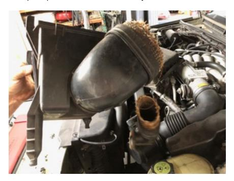
Remove the Genuine Land Rover Rat's nest at air box and fender elbow sides If you are planning on doing water crossings it is advisable to use some silicone based sealant to plug up this hole on the lower airbox lid. Two attached photos show the outside and inside position.
